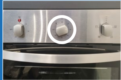
Step 2: Turn the timer to set the length of time you'd like to use the oven.
